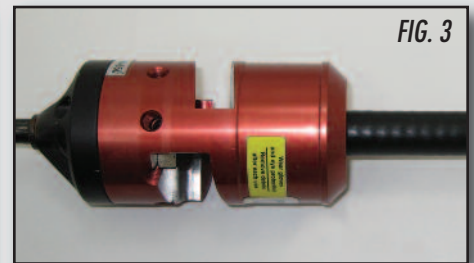
Install the 123-1AS into a standard drill and strip the cable.
